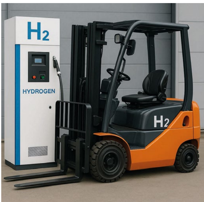
Figure 1: Fuel cell-powered forklift next to a hydrogen dispenser.
